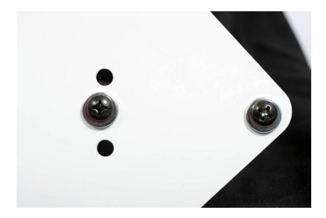
3. Place the flat washers on the four <sup>1</sup>/<sub>4</sub>"-20 screws and insert them into the desired yoke holes. Place one rubber washer on each screw, inside the yoke, just enough to hold the screws in place. (See photo below.) This will also keep the rubber washers in place when sliding the cabinet into the yoke.
