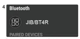
In your Bluetooth® enabled device, scan for devices and locate the JIB/BT4R. Tap it to connect to the receiver.
