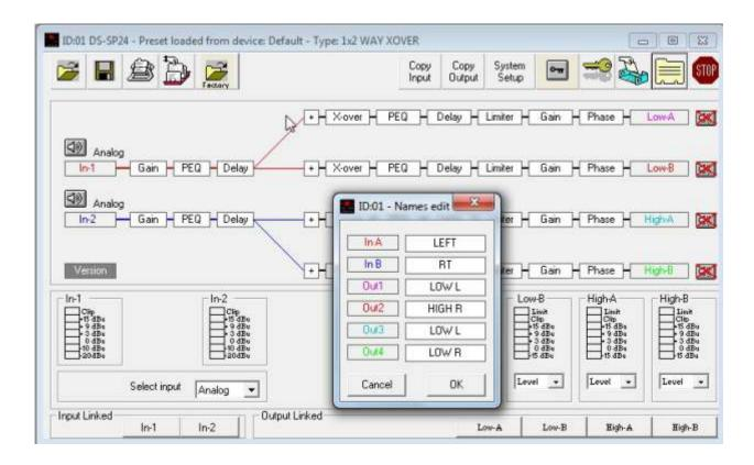
Select the gain block to access the gain and polarity of the inputs and outputs.
