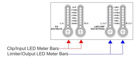
**LED Meter Bars for the Clip/Input** - these bars of LED meters indicates, when turned on, clipping of the input signal, with the other LEDs showing the current input level BEFORE ANY PROCESS, ranging from +20dBu (Clip) up to -20dBu.
