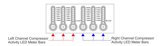
**LED Meter Bars for the Compressors Activity** - these bars of LED meters shows from top to bottom, the activity of the RMS Compressors.
