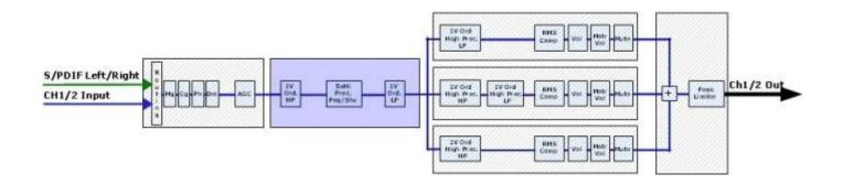
**HPF sub-menu** - from this sub-menu, it is possible to set the Input Channels High Pass Filter (HPF), preceding the bank of 5 Peaking/Shelving filters.
