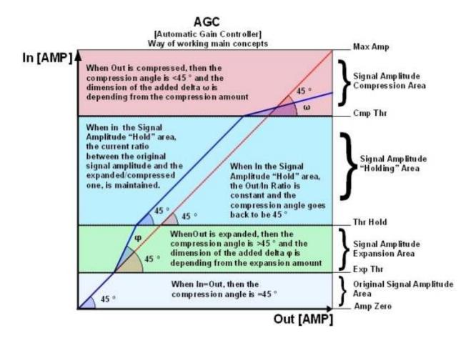
The AGC is an Expansion/Compression process applied with slow Attack and Release times, to the INPUT signal of a Unit, in order to maintain the average amplitude of the OUTPUT signal at a defined level, independently from the average amplitude of the input sources.
