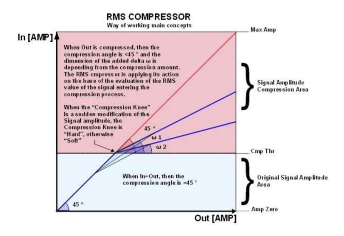
The RMS Compressor is a Compression process, applied with fast slow Attack and Release times to the INPUT signal of a Unit, in order to maintain the amplitude of the OUTPUT signal at a defined level, when input level is exceeding a defined intervention Threshold.
