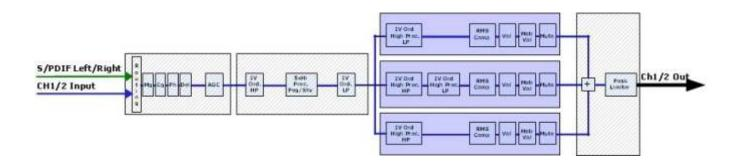
The DS-CP25 multi band compressor, can operate as 3 bands, 2 bands or Mono band compressor unit. Because of that, within the Compressors Menu there are up to 3 common control pages, allowing the user to set the number of bands for the compressor and, independently from this selection, to set the X-Over frequencies for the definition of the 3 or 2 bands.
