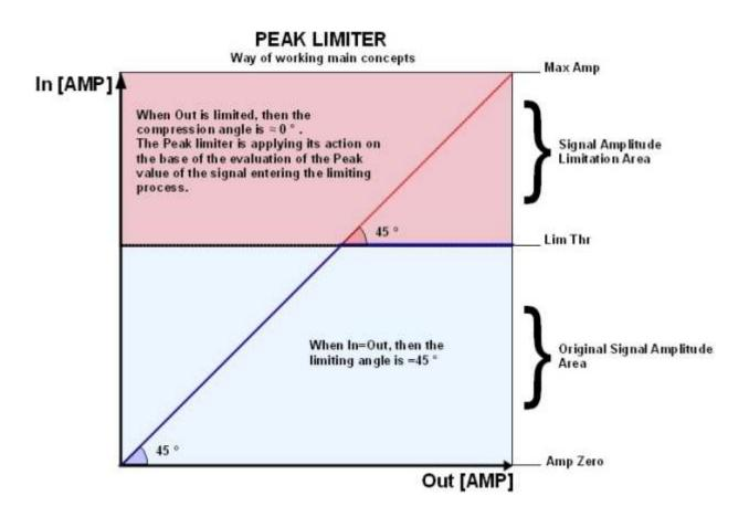
This kind of Limiter, as illustrated by the picture here above, is useful for the amplifier's and Loudspeakers' protection.
