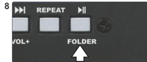
8 MP3 Player Play/Pause/Folder: Pressing Play/Pause will either play or pause the audio. Press and Hold the button for the Folder function. You can switch between folders in a USB device.
