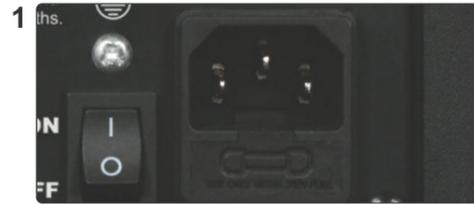
1 Connect power cable to TQ6, connect other end to a power outlet to charge immediately. Once charged, the TQ6 can be operated on AC or Battery Power.
