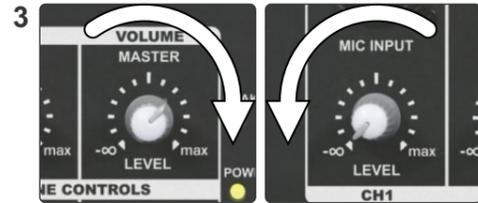
3 Level control: Use the Channel Level control to raise your input to the desired level. If needed, the Master Level can be raised.
