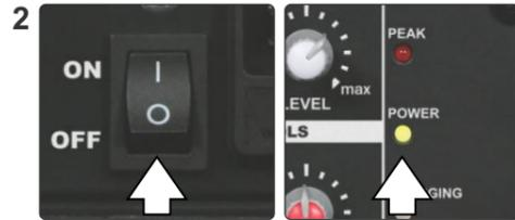
2 Power on the TQ6 by pressing the power switch into the ON position. The Power LED will light up.
