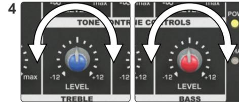
4 To adjust the Treble, turn the knob clockwise to increase or counter-clockwise to decrease. To adjust the Bass, turn the knob clockwise to increase or counter-clockwise to decrease.
