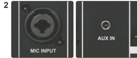
2 Connect your microphone to CH1 with an XLR or 1/4" Cable, or connect an 1/8" Cable source to the CH2 AUX input.
