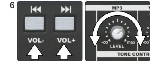
6 MP3 Player Skip/Volume: Skip forward or backward between tracks by pressing the skip buttons. Holding the buttons down will increase or decrease the volume. The level is also controlled by the MP3 Level knob.
