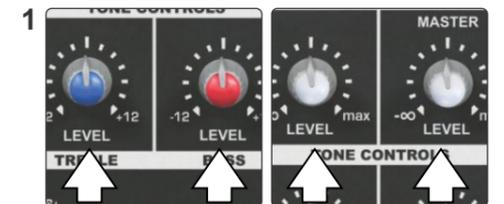
1 Start with the Master Level, Treble, and Bass controls set mid-way. All other level controls should be turned down (counter-clockwise to lower, clockwise to increase).
