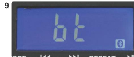
9 MP3 Player Bluetooth: In Bluetooth mode, pairing is activated. Make sure your Bluetooth enabled Smart Device is on. Find the TQ6 in the device list, then select it to pair.
