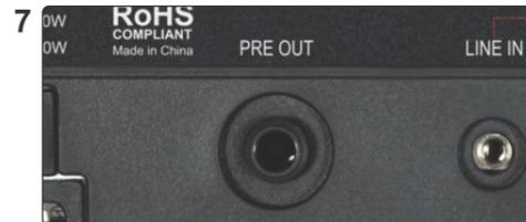
7 The Pre Out provides a Line Level mix of all three channels.
