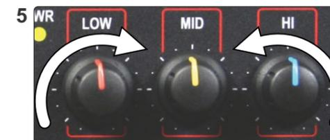
5 EQ controls - Low/Mid/Hi: To increase the low, mid, and high frequencies, turn the appropriate tone control clockwise. To decrease, turn counter-clockwise.
