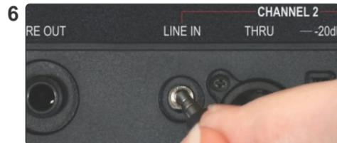
6 For a stereo signal from an MP3 player, attach 1/8" stereo cable into the Channel 2 1/8" input.
