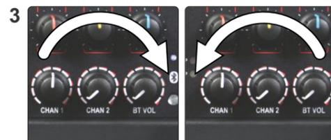
3 Level controls: turn clockwise to raise the level. Turn counter-clockwise to lower the level.
