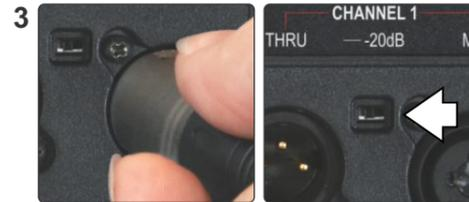
3 For a balanced mic signal, plug the XLR male end of the cable into the XLR/1/4" Combo Input on the PA6BT. For strong signals, engage the -20dB Pad Switch to prevent distortion.
