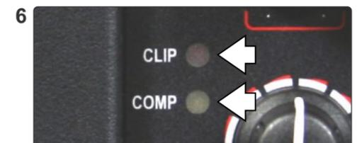
6 Reduce Input Levels if the Clip LED turns on. Max. level is reached when the yellow "Comp" light flashes at peak levels. If the light is on constantly, turn the levels down to avoid damage to the PA6BT.
