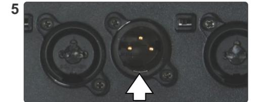
5 Connect a female XLR to the Thru output to feed the channel's XLR input to another device.
