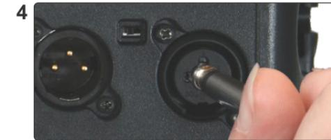
4 For Balanced or Unbalanced Line Level, plug the 1/4" cable into the XLR/1/4" Combo Jack on the PA6BT.
