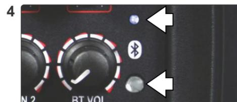
4 Using Bluetooth® - Press the Bluetooth® button. The Bluetooth® LED will flash for 15 seconds. Locate the PA6BT on your device and select to pair. If pairing fails, turn Bluetooth® off and try again. The button also acts as a Stop/Play/Pause. Powering the unit off will disconnect.
